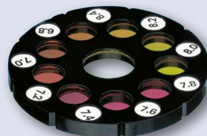
Test disc with colour stable glass standards
