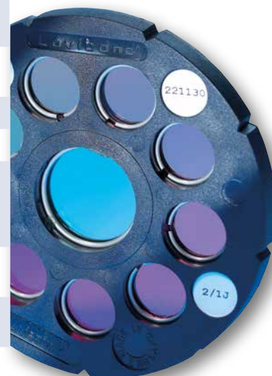
Test disc with colour-stable glass standards
