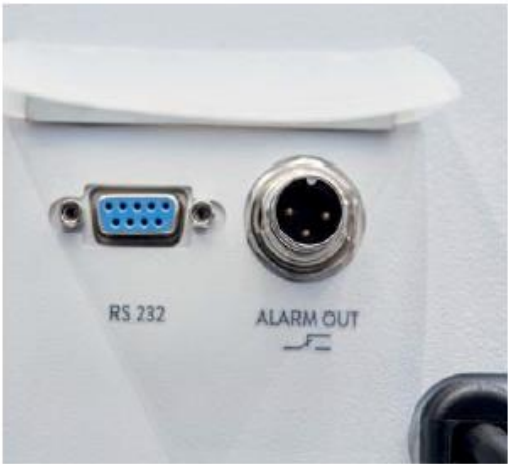
Standard-issue RS 232 interface and alarm contact
