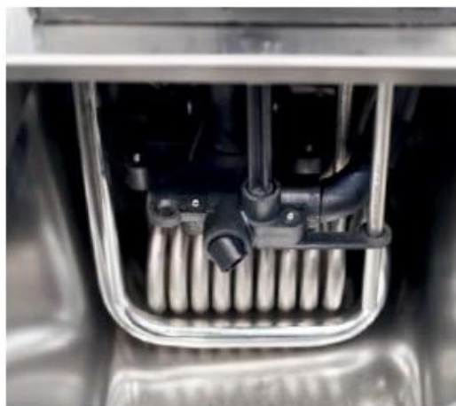
Standard-issue cooling coil included with all heating thermostats
